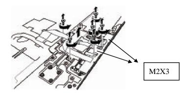
Figure 4-21 Removing the bracket
